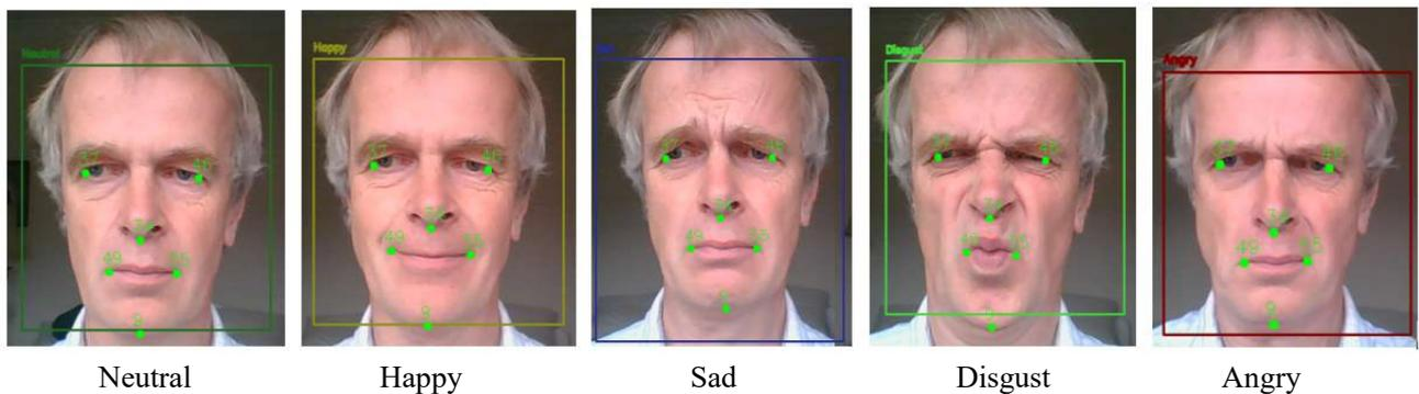
**Figure 3: Diagnostic display showing 5pt facial landmarks attached to face and emotion estimate based on five acted facial expressions.**
