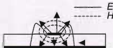
Fig.2.24: Electric and magnetic field lines of a Microstrip line
