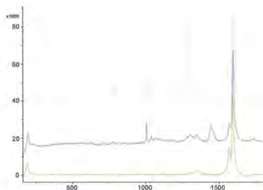
Figure 3. Raman Spectra of tubes, terphenyl tube mixture and raw terphenyl
