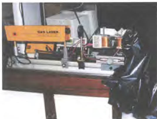
Figure 2. Apparatus showing laser (left) followed by polariser and magnetic poles (right)
