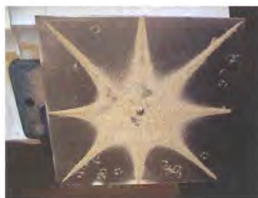
Figure 4. Mode of frequency 643Hz - bow experiment.
