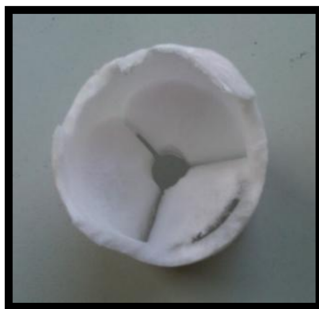
Figure 3. The image above shows the CG freeze dried construct. Through optimisation of the freeze drying process, a tri-leaflet valve was fabricated.
