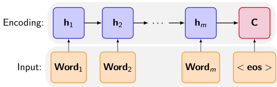
Figure 11: Using an RNN to Generate an Encoding of a Word Sequence: the symbol  $\langle eos \rangle$  is a special symbol used to mark the end of a sequence, the box labelled **C** holds the embedding for the word sequence.
