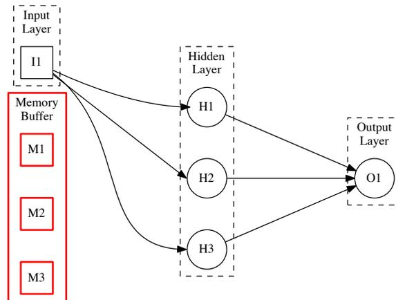
Figure 5: Adding a memory buffer to a feed-forward neural network with one hidden layer
