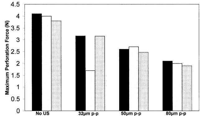
Fig. 5. Maximum penetration force (through intima-media layer) with no ultrasound applied (No US) and for ultrasonic wire waveguide distal-tip displacement of 32, 50 and 80  $\mu\text{m}$  peak-to-peak. All 12 tissue tests shown. Waveguide feed-rate = 0.5 mm/s.
