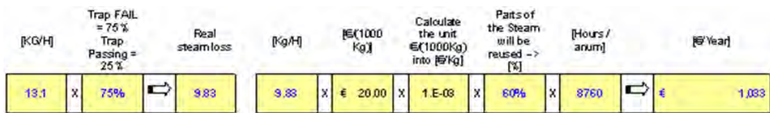
Figure 4.10 Steam loss calculation for failed steam traps
