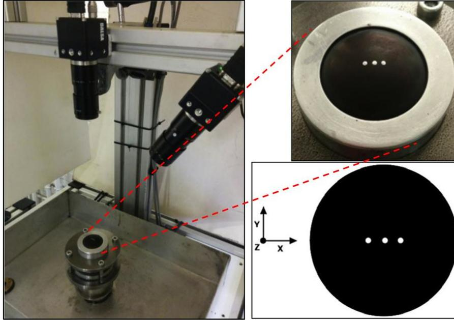
Fig. 2 Inflation orifice for bubble inflation test
