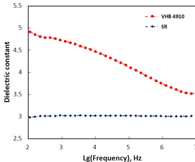
Fig. 3 Plots of dielectric constant versus frequency
