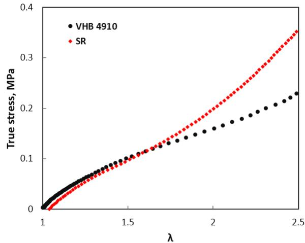
Fig. 4 The relation between true stress and stretch ratio
