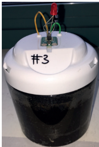
Figure 1: The Mudwatt MFC that was used over the course of this study.
