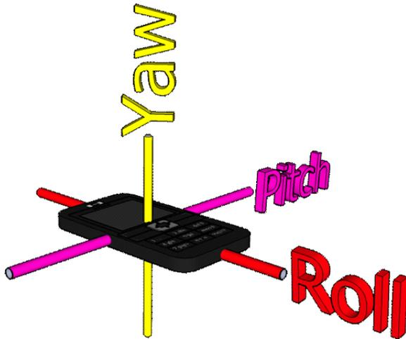
Figure 1: Roll, Yaw and Pitch axis.
