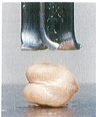
Fig. 3.4. Sample orientation during compression testing.
