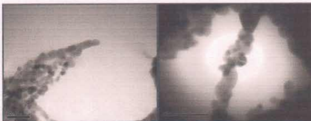
Figure 13 TEM images at 200000x of powders made from solutions containing 1mmol zinc acetate and (l) 15mmol acetic acid, (r) 87mmol acetic acid, calcined to 500°C
