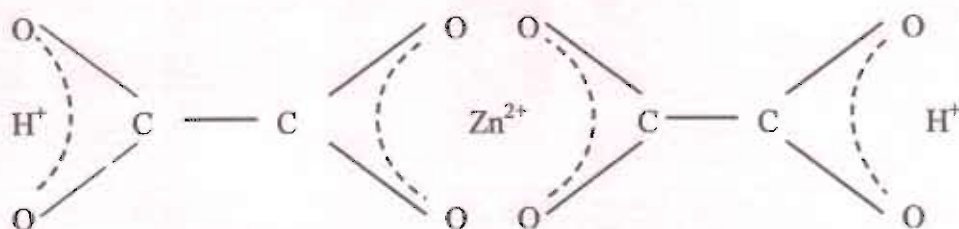
Figure 4 Schematic of precursor proposed to have formed under rapid combination of reagents
