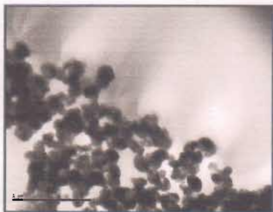
Figure 20 TEM image of powders synthesized in a 1:100 ratio with isophthalic acid and sintered to 800°C, 40000X
