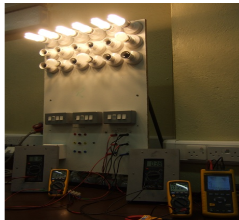
Figure 20. Neutral and phase current measurement for a 3 phase balanced CFL load
