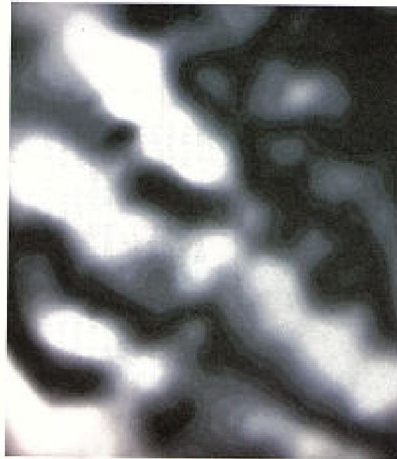
Fig. 22. First derivative gravity image (gradient), showing NE trending derivative highs which correspond to major NE faults. [Photography by Condt. Patrick Walshe (Retd.)]
