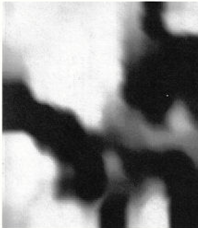
Fig. 20. Grey scale Group Mean image of serial photograph lineaments between 60 and 100 degrees. In light toned regions, lineaments strike close to 100 degrees, in dark toned areas they strike near to 60 degrees. NE trending light zones follow trend of dextral wrench faults. [Photography by Comdt. Patrick Walshe (Retd.)]
