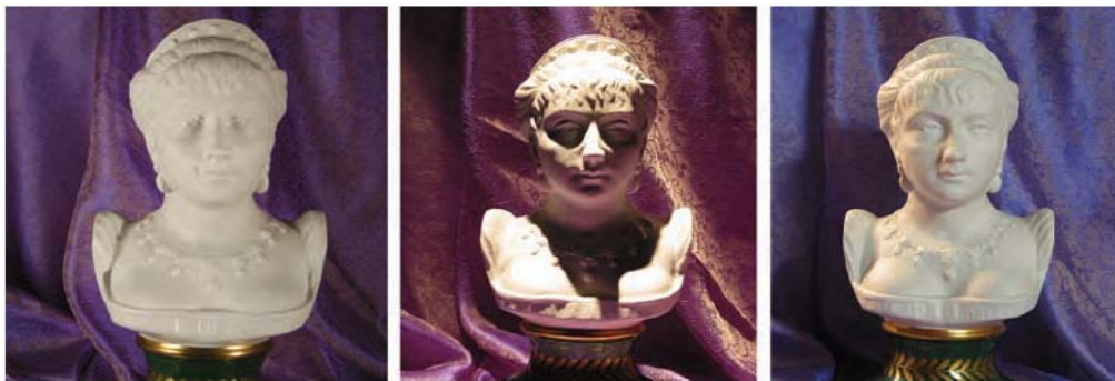
Fig 2: Modelling of a bust by different light distributions. From left to right, lighting is completely diffuse, strong down-lighting and a combination of directional and diffuse lighting [2]
