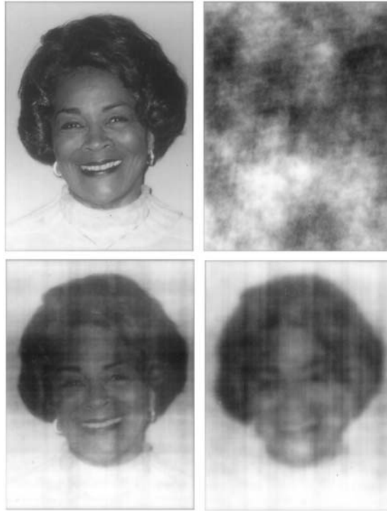
Figure 11.9: Original (top-left), diffused watermark (top-right), reconstruction using a flatbed scanner (bottom-left) and reconstruction using a mobile phone (bottom-right). These images have been scanned in grey scale from the original colour versions printed on to a personal ID card at 600dpi stamp-size (i.e. 2\text{cm} \times 1.5\text{cm} ).
