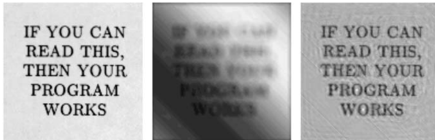
Figure 12.6: 128 \times 128 test image (left); non-stationary convolution of test image using a tophat PSF with energy conservation where the average tophat half-width is 4 pixels (centre); restoration of the image using the conjugate gradient method (right).
