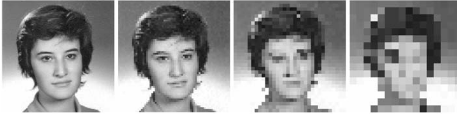
Figure 2: A digital image sampled using (from left to right) 128 \times 128 , 64 \times 64 , 32 \times 32 and 16 \times 16 pixels.
