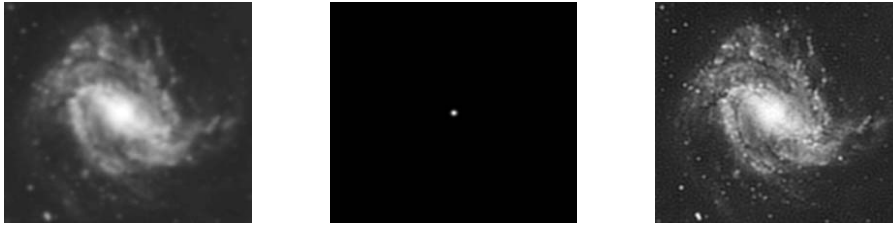
Figure 12.1: Example of the application of the Wiener filter. Original image (left), Gaussian point spread function (center) and restoration after application of the Wiener filter (right) using a standard deviation of 3 pixels and SNR=1.
