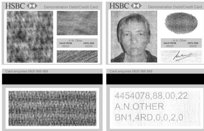
Figure 11.8: Example of the application of ‘diffusion only’ watermarking. In this example, four images of a face, finger-print, signature and text have been diffused using the same noise field (with pre-processing) and printed on the front (top-left) and back (bottom-left) of an impersonalized card using a 600 dpi printer. The reconstructions (bottom-left and bottom-right, respectively) are obtained using a conventional flat-bed scanner based on a 300 dpi grey-level scan.
