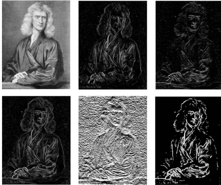
Figure 16.3: An image of Isaac Newton (top-left), D_x (top-centre), D_y (top-right), G = |D_x| + |D_y| (bottom-left), \tan^{-1}(D_y/D_x) (bottom-centre) and G after binarization with threshold = 0.2 (bottom-right).
