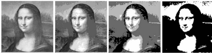
Figure 3: A 128 \times 128 image with luminance quantization using (from left to right) 4, 3, 2 and 1 bits.
