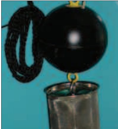
Fig. 2.6 Floating suction filter installed on submersible pump.
