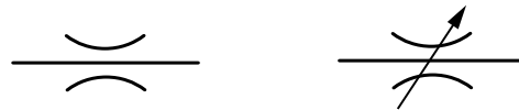
Figure 6-1 Symbols for a fixed area flow restrictor and a variable area flow restrictor
