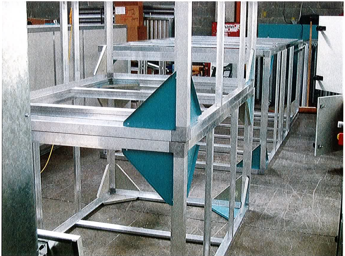
Fig. 23: Typical Frame Construction for Air-Handling Units
