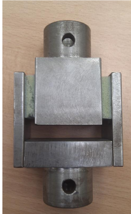
Fig.3 Shear test set-up, left hand side sample failed due to shear
