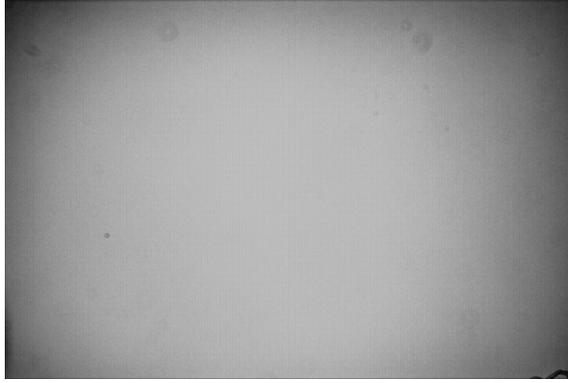
**Figure 2.3:** Example of a flat field Image.
