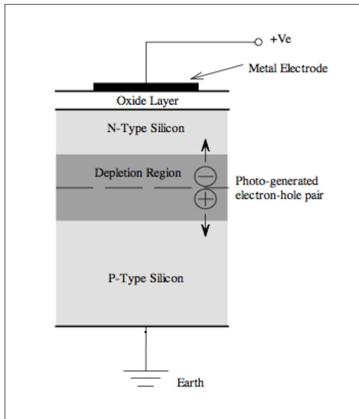
**Figure 1.5:** Cross section through a CCD pixel [23].
