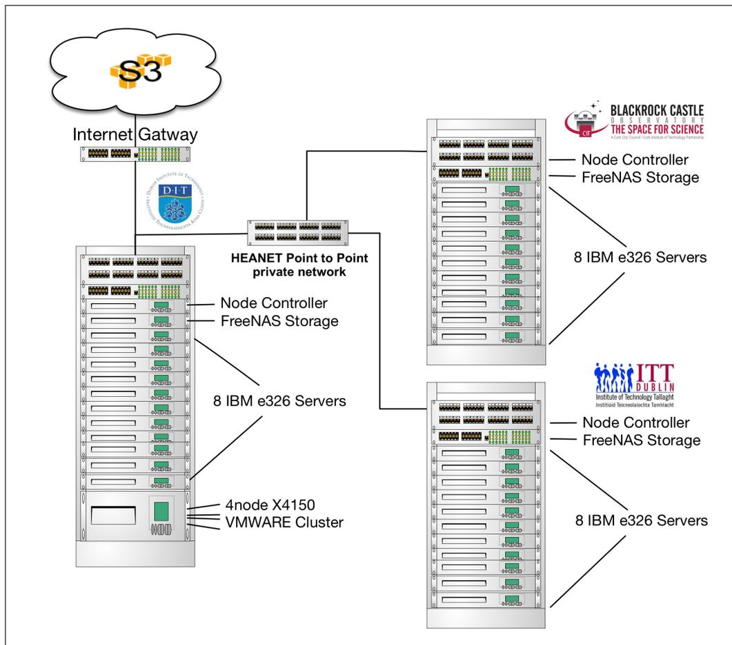
Figure 4.2: ACN network diagram connecting multiple institutes.
