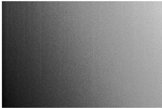
**Figure 2.2:** Example of a master bias frame.
