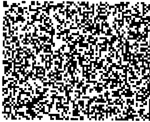
Figure 1.1: The image above shows an example of a typical data page. This one consists of 60 x 80 bits represented by bright and dark squares.
