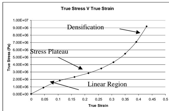
Figure 2: True stress-true strain curve from compression testing
