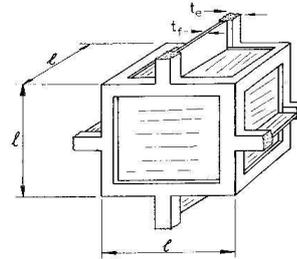
Figure 4: Closed cell foam [4]
