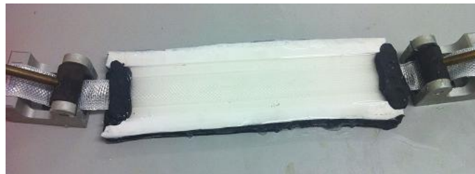
Figure 2. The fibre tape was clamped at both ends of the mould.
