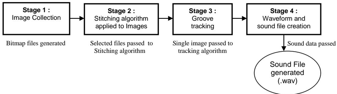
Figure 2: Stages in development of optical playback process
