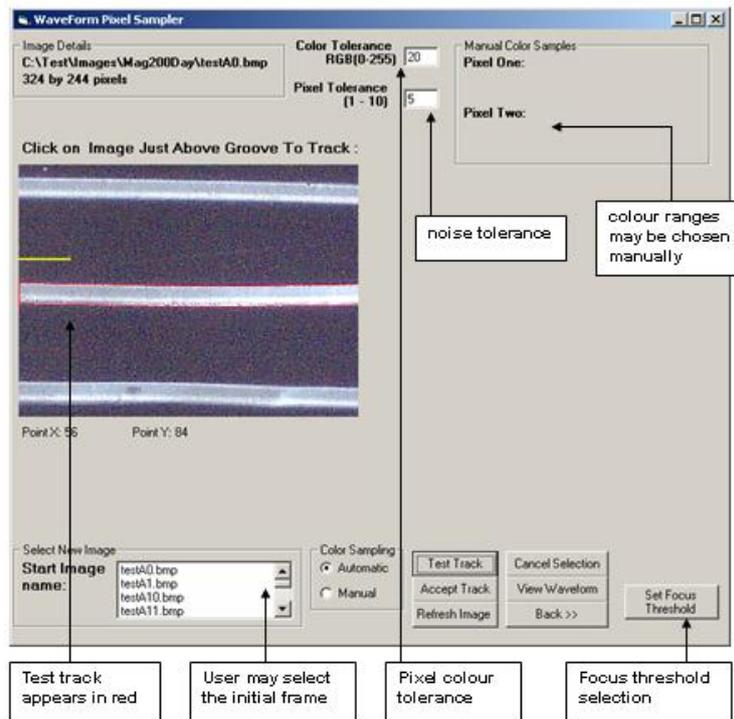
Figure 10: Groove tracking process
