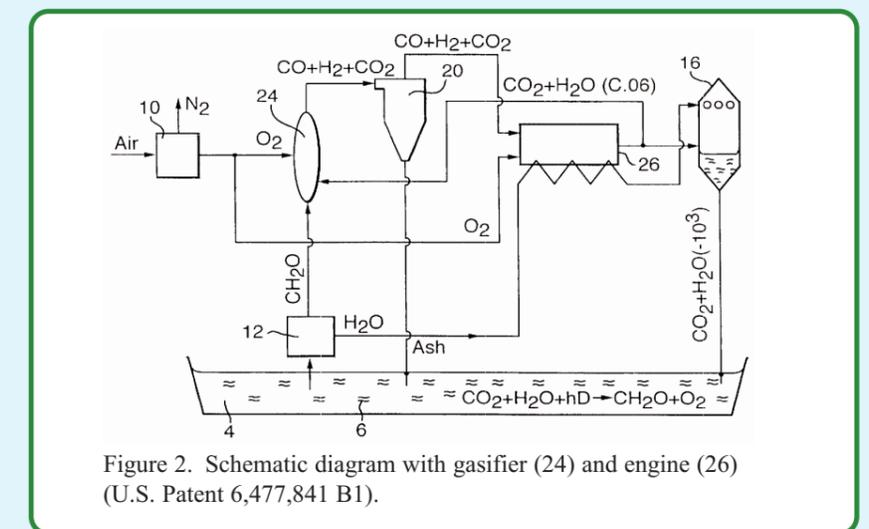
Figure 2. Schematic diagram with gasifier (24) and engine (26) (U.S. Patent 6,477,841 B1).
