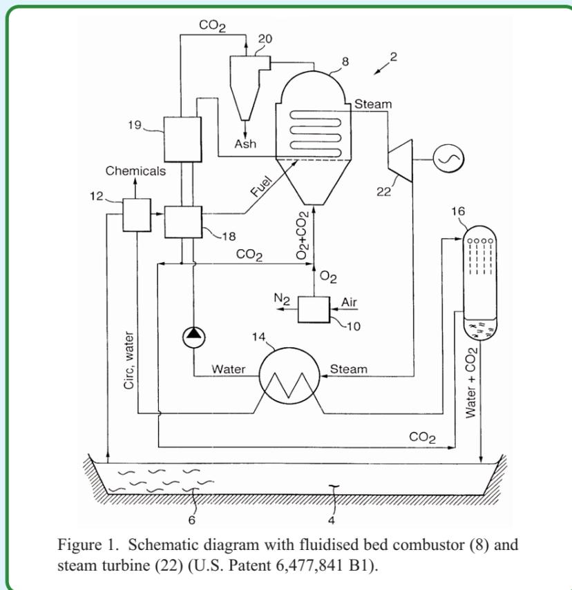
Figure 1. Schematic diagram with fluidised bed combustor (8) and steam turbine (22) (U.S. Patent 6,477,841 B1).
