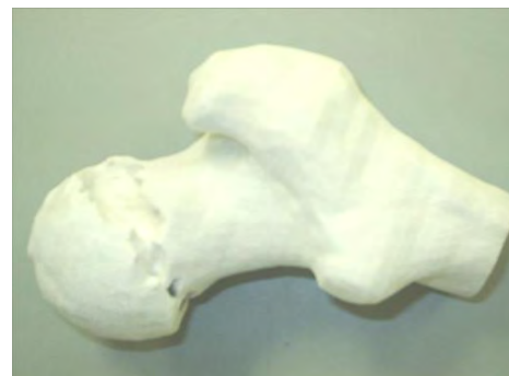
Figure 9.52 (a), (b) Z-Corp model of pelvis and femur head.
