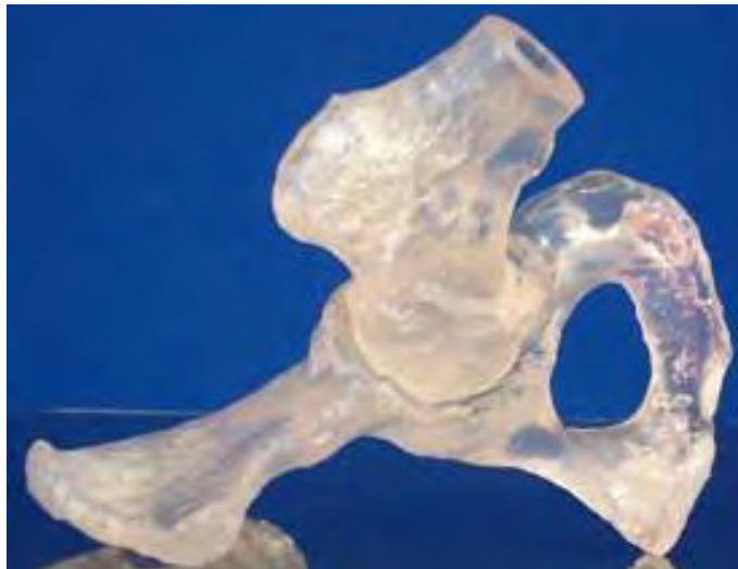
Figure 4.6 A 3D SLA model of a pelvis and femur. [57]
