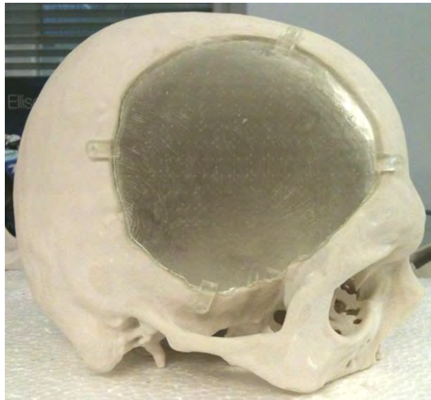
Figure 9.36 Completed skull model produced on Z-Corp 3D printer and cranial plate model produced on EOS 250 SLA RP machine.
