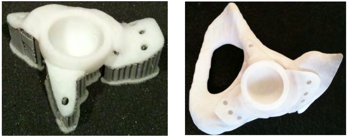
Figure 9.84 (a), (b) Acetabular cup model implant shown with support material on FDM machine. Pelvis 3d printer model with acetabular cup model assembled.
