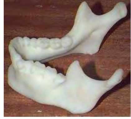
Figure 3.8 [36] and 3.9 [37] components manufactured by the FDM process.
