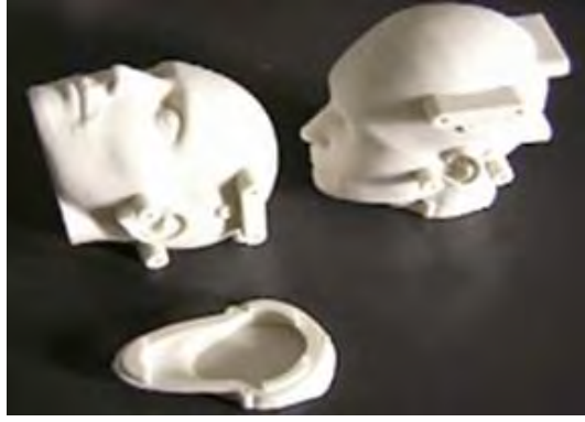
Figure 3.8 [36] and 3.9 [37] components manufactured by the FDM process.
