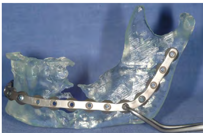
Figure 4.3 SLA model of a mandible bone fitted with a customised implant. [54]
