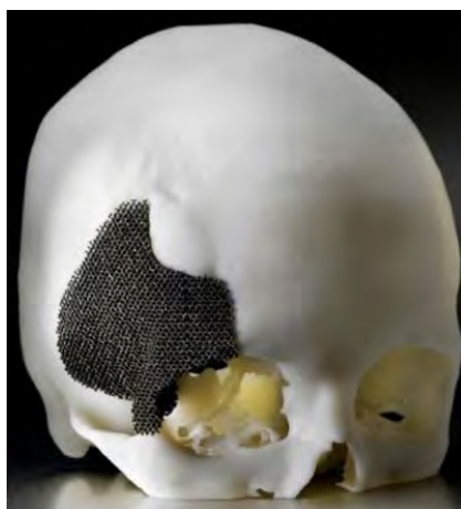
Figure 3.13 Skull model used for placement and fit of implant. [43]
