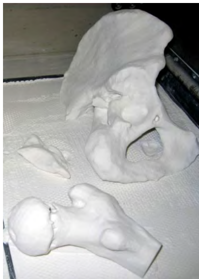
Figure 9.51 Pelvis, femur and fragment built on Z-Corp 3D printer.
