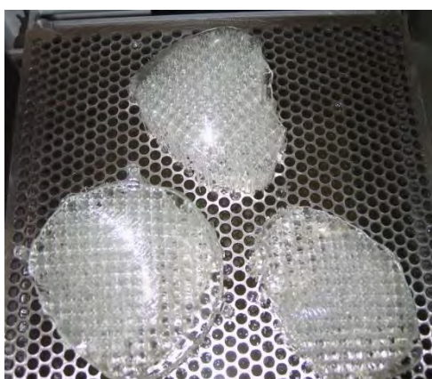
Figure 9.10 Cranial plates rapid prototyped on 3D Systems 250 SLA machine.
