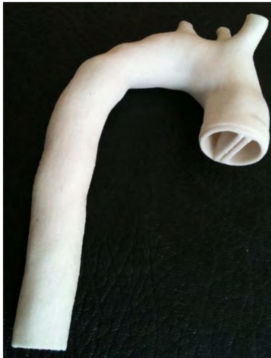
Figure 9.114 Combined Z-Corp RP model of aorta and heart valve.
