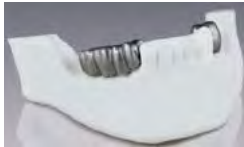
Figure 3.6 A Direct Metal Laser Sintering (DMLS) dental implant fitted to a SLS mandible model. [33]
