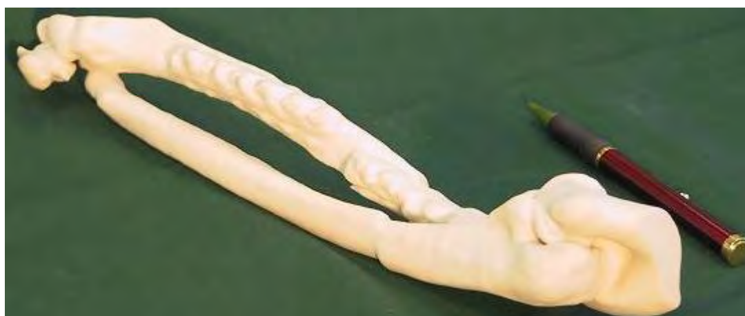
Figure 4.7 A right forearm FDM model with a broken radius bone. [58]
