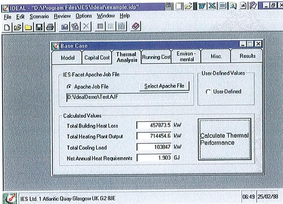
Figure 7.7: Thermal Calculation tab.
