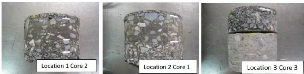
103 Figure 2. Cores taken from existing pavement showing a large variation in material present
