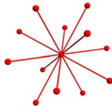
Figure 1. The central joint with twelve equally distributed spokes is a gusset. Alexander Graham Bell used gussets of this type to build structures, including many kites. Replication of the gusset and the links between gussets gives rise to cuboctahedral trusses, structures and space frames, which in engineering terms can be strong, rigid and light.
