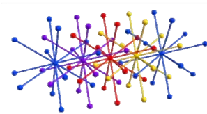
Figure 38 Node gussets (or joints) from four Bell Fuller lattices forming a line of nodes of the composite 4-colour lattice 12 . The two blue gussets are from the same Bell Fuller lattice.
