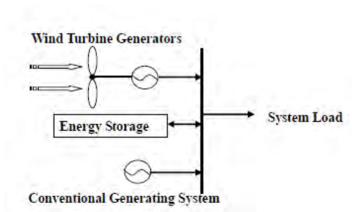
**Figure 11: Model of System with Energy Storage**
