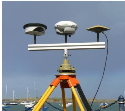
Fig. 5: Bracket allowing simultaneous observation with three receivers.
