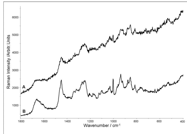
Fig.1: Examples of Raman spectra collected from human skin sections dry (A) or immersed in water (b) using a 785 nm wavelength. Spectra result from 1 x 10s acquisitions. No pre-processing or offset have been applied to the spectra.
