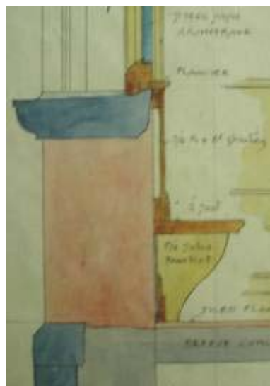
Figure 5/49 – Enniscorthy P.O., c.1910; Section through Seat in Public Office 191
