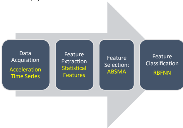
Figure 1. Summary of damage detection approach
