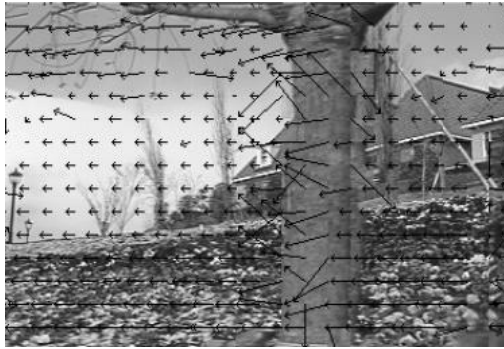
Fig. 4.7 The Flower Garden sequence with its Motion Vectors overlaid. The Flower Garden sequence involves a pan from left to right, a motion vector points to the best match macroblock in the reference frame, hence the predominance of motion vectors pointing to the left. Source: Girod, (2008).
