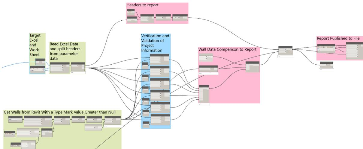
Fig. 9: Script 2 - Information Verification and Validation - Wall Types
