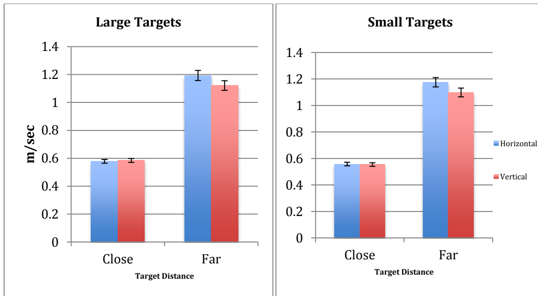
Figure 3: Peak Velocity Values shown for both horizontal and vertical orientations when the targets were close and far when the Target Width was large (A) and small (B) in both horizontal and vertical conditions.
