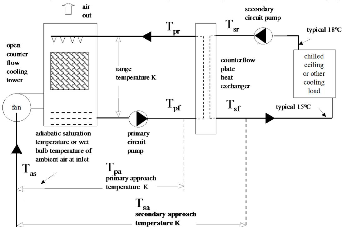
**Figure 1. Simplified schematic of an indirect evaporative cooling system (IDEC)**
