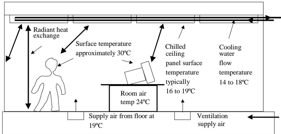
**Figure 3. Principle of radiant cooling by chilled ceilings**
