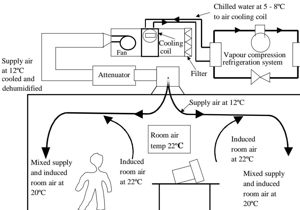
**Figure 2. Traditional (all air) air conditioning cooling system**
