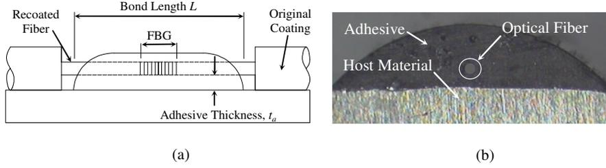
**Fig. 2.** (a) Surface bonded FBG sensor (b) View of the optical fiber within the adhesive layer
